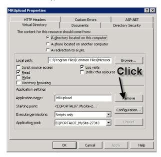
Figure 58: Removing the MRUpload application
